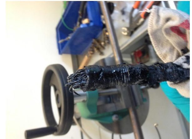
Figure: Polymerization of biocrude observed in a pilot plant unit
