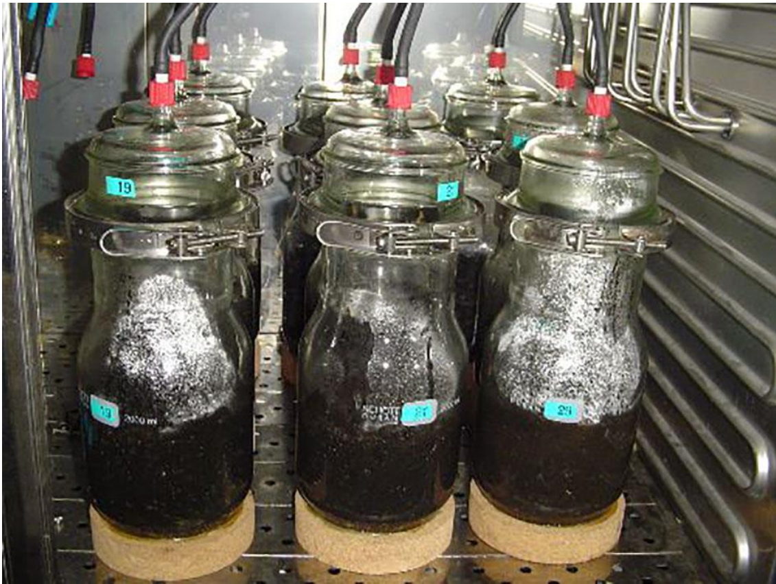
Picture 3: Anaerobic digestion for biogas production. © OWS
